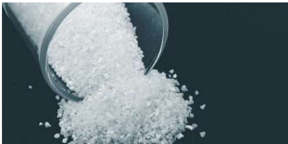
Figure 1: MCD Apatitic Abrasive, a multi-phase calcium phosphate principally composed of hydroxyapatite and tricalcium phosphate, is manufactured directly by Himed and available globally for MATRIX MCD® grit-blasting applications.
